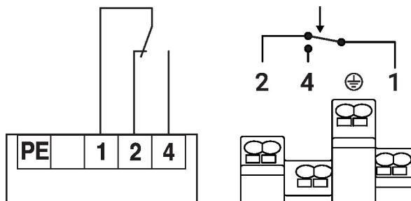
If the capillary leaks, the electrical circuit 1-4 is permanently closed. Unlocking is no longer possible.
