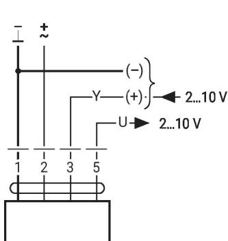
Override control (frost protection circuit)
