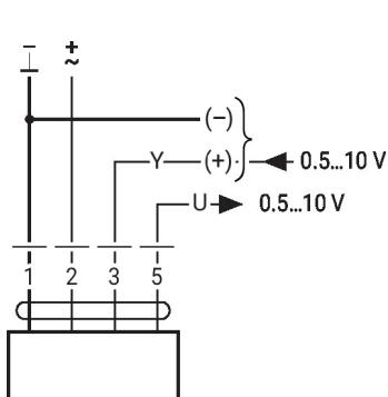
Override control (frost protection circuit)
