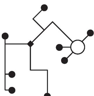
There are no restrictions for the network topology (star, ring, tree or mixed forms are permitted). Supply and communication in one and the same 3-wire cable
