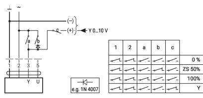
Control remotely 0...100% with positioner SG..
