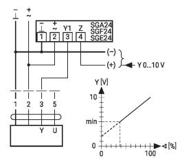
Override control with AC 24 V with rotary switch
