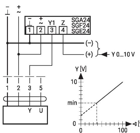
Override control with AC 24 V with rotary switch
