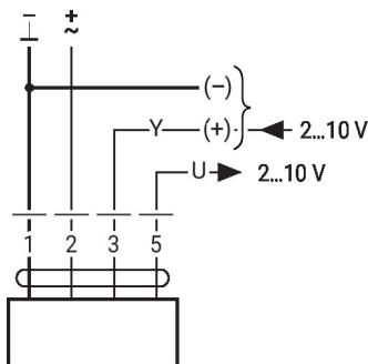
Override control (frost protection circuit)
