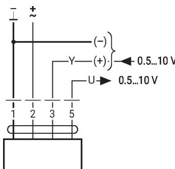
Override control (frost protection circuit)
