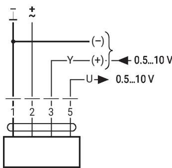
Override control (frost protection circuit)
