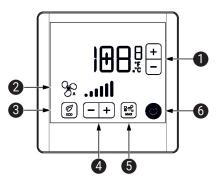
Temperature setpoint: Set the desired temperature
