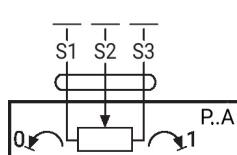
Recommendation: wiring as a voltage divider
