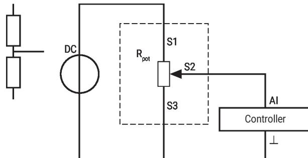
If the potentiometer is mainly operated in the same small angle range, we recommend wiring it as a voltage divider.
