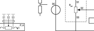
If the potentiometer is mainly operated in the same small angle range, we recommend wiring it as a voltage divider.
