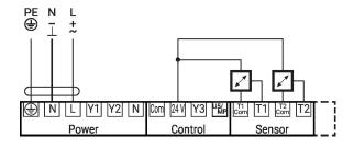
Switching contact connection (BACnet MS/TP / Modbus RTU)
