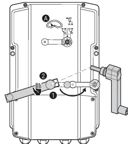
For the auxiliary switch position settings, carry out points 1 to 4 successively.
