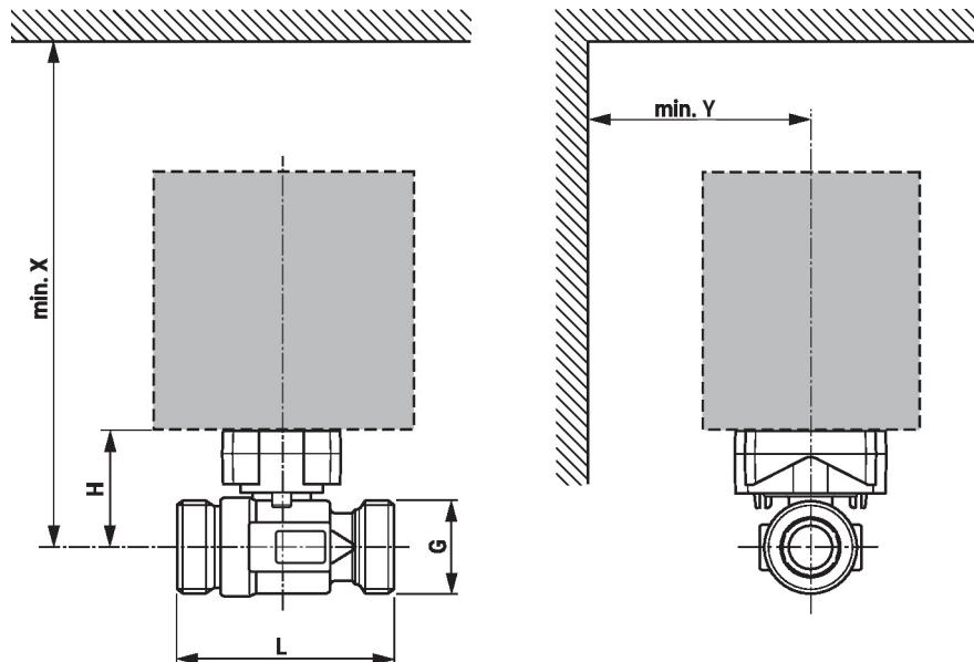
X/Y: Minimum distance with respect to the valve centre.
