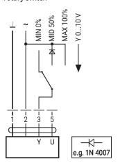
Control remotely 0...100% with positioner SG..
