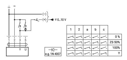
Override control with AC 24 V with rotary switch
