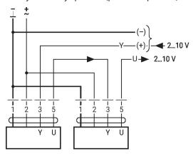
Control with 4...20 mA via external resistor
