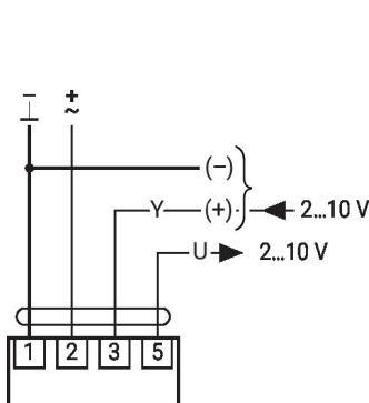
Override control (frost protection circuit)
