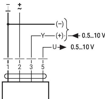
Override control (frost protection circuit)
