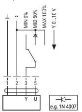
Control remotely 0...100% with positioner SG..
