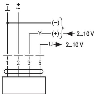
Override control (frost protection circuit)
