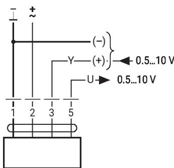
Override control (frost protection circuit)
