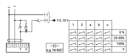
Override control with AC 24 V with rotary switch
