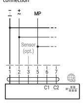
MP-Bus via 2-wire connection, local power supply
