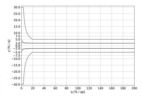
— Water ---- Water + Glycol (≤60% Glycol) y = Measuring accuracy q = Measured flow qp = Nominal flow
