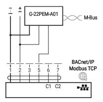
M-Bus parallel Modbus RTU or BACnet MS/TP
