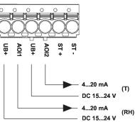
Correct temperature values are only available, when the humidity output AOI1 and both inputs UB + are connected.
