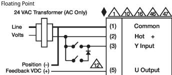
VDC/mA Control 24 VAC Transformer (1) Common Line Volts (2)Hot + 500 Ω 1/4 watt Control Signal (-) VDC/mA (+) (3) Y Input Position (5) **U** Output Feedback VDC
