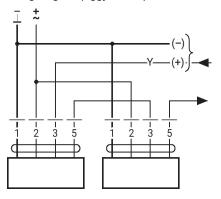
Max. 2 actuators in primary/ secondary operation Primary/secondary operation is permitted only on one fixed shaft or on two mechanically coupled shafts The programming of the primary actuator is adopted by the secondary actuator
