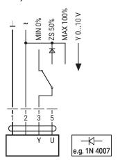
Control remotely 0...100% with positioner SG..
