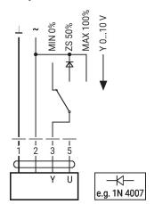
Control remotely 0...100% with positioner SG..
