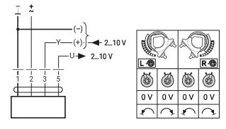
Wiring diagram piggy-back operation (mechanically coupled actuators)
