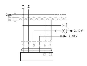
MP-Bus, supply via 3-wire connection
