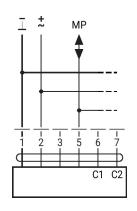
MP-Bus via 2-wire connection, local power supply
