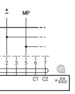
MP-Bus via 2-wire connection, local power supply
