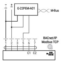
Examples of external wiring with actuator types ..24GX..
