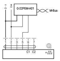
M-Bus with converter in parallel mode with PoE with BACnet/IP / Modbus TCP  $\,$
