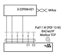
M-Bus with converter in parallel mode with BACnet/IP / Modbus TCP
