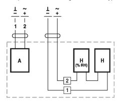
A = Actuator H [% RH] = Humidistat H = Heating
