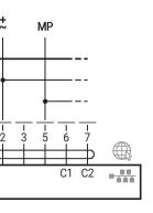
MP-Bus via 2-wire connection, local power supply
