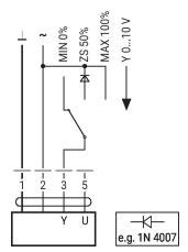
Control remotely 0...100% with positioner SG..
