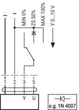
Control remotely 0...100% with positioner SG..
