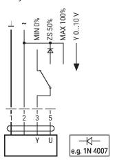
Control remotely 0...100% with positioner SG..
