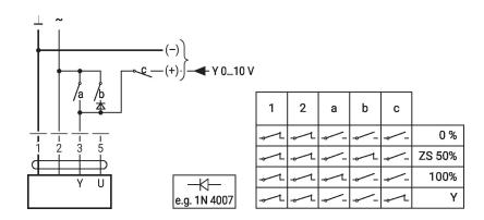
Override control with AC 24 V with rotary switch
