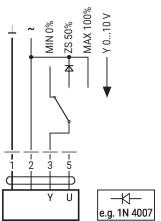
Control remotely 0...100% with positioner SG..
