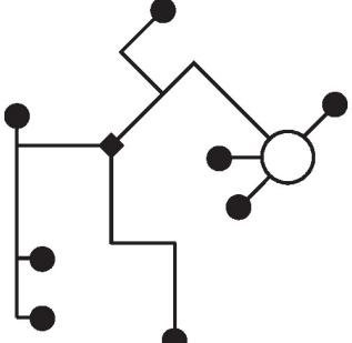
There are no restrictions for the network topology (star, ring, tree or mixed forms are permitted). Supply and communication in one and the same 3-wire cable
