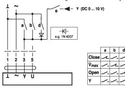
Override control and limiting with DC 24 V with relay contacts
